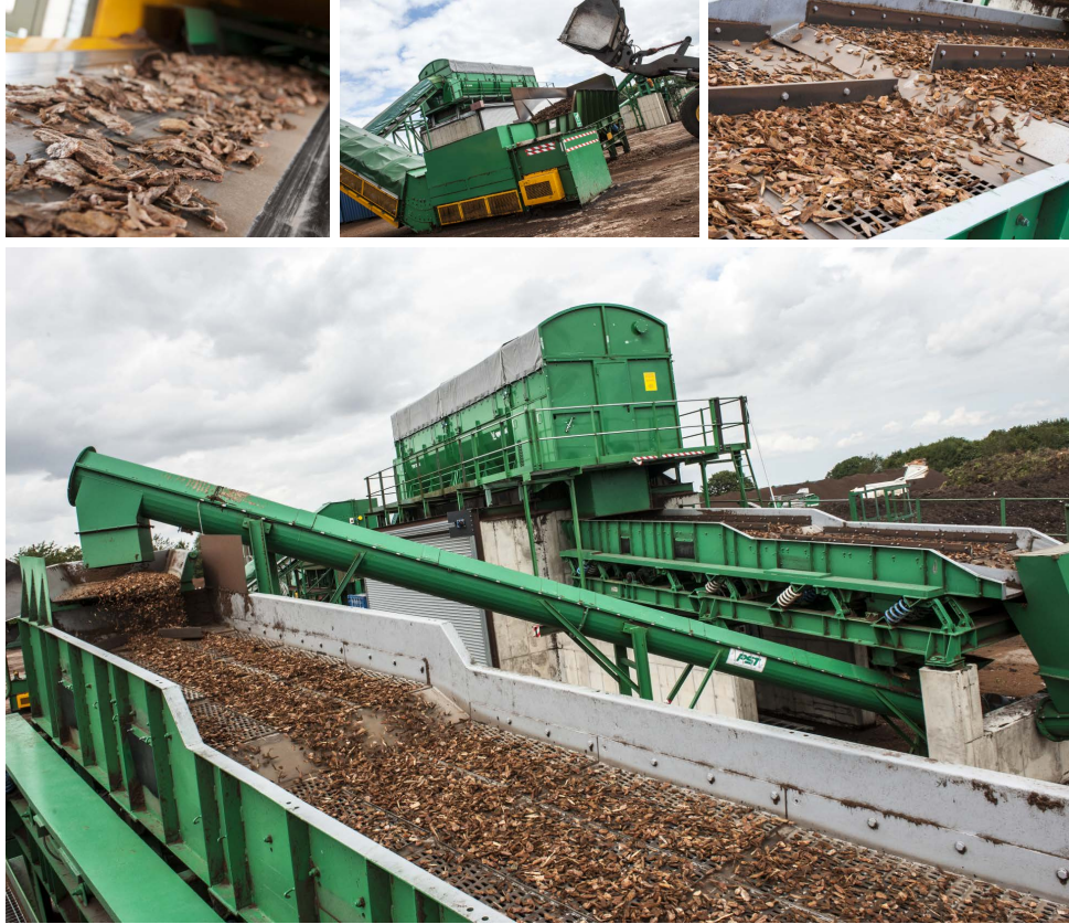
TMA Bark's new custom designed and built production plant processing raw bark material to produce the new pure range of products.
